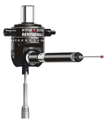
RTP20 integral TP20 probe mount optimises the working volume of the CMM and provides compatibility with all existing TP20 modules. Although modules can be changed manually, the RTP20 can be used with the MCR20 module change rack, allowing fully automated module changing.
